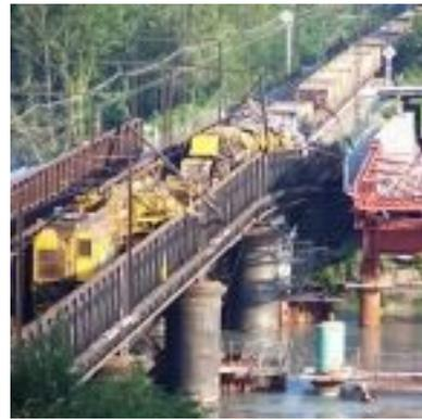
*On Monday 24 July 2006, at about 6:30 p.m., the works train 818 729 was running from the station at Culoz (its base) towards the track replacement worksite of Moirans-Grenoble. During the acceleration of the train, as it was passing through the passenger station at Culoz, the "working group" was derailed. This "working group" is the unit that removes old sleepers, lays new sleepers and levels the ballast, which is supported on the track by a deballasting axle.*
