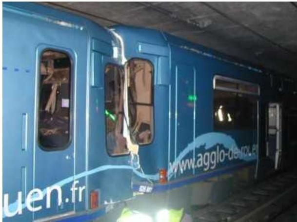
The Rouen tramline includes an underground section, equipped with a block signalling system similar to that on an underground railway. On the morning of 30 August 2004, a tram set wrongly crossed a signal light set at stop and collided with the rear of a tram stopped ahead of it in the tunnel.
