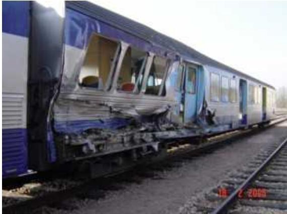
On 16 February 2005, train 117710 from Provins (Seine and Marne) was in a broadside collision with train 117578 at Longueville station (Seine and Marne). By chance, there were no casualties; only equipment was damaged (leading coach of the buffered train was smashed open, miscellaneous damage to the body of the locomotive, distortion of the track and the adjacent platform).
