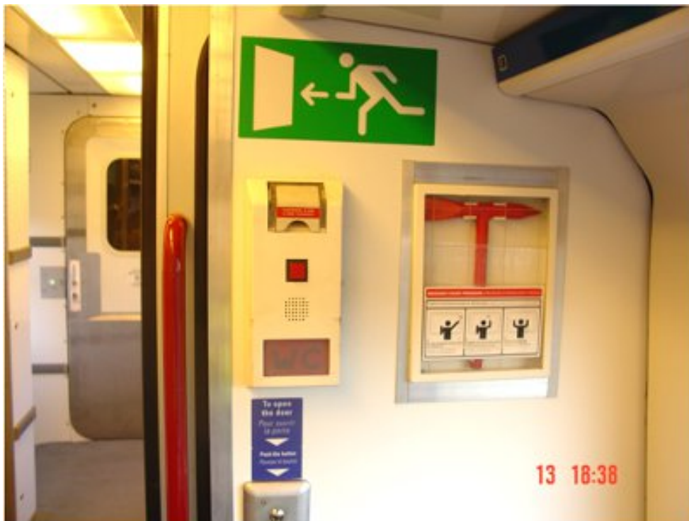
Figure 25: Amenity coach, hammer for breaking windows
