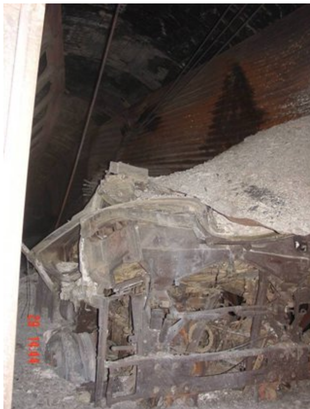
Figure 34: Damage suffered by one of the carrier wagons and its load
